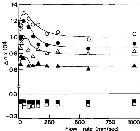
**Figure 8** Birefringences (at  $r/r_0 = 0.5$ ) of transverse (circles,  $\Delta n \equiv \Delta n_{yx}$ ) and longitudinal (triangles,  $\Delta n \equiv \Delta n_{zx}$ ) cut sections and as-formed cylinders (squares,  $\Delta n \equiv \langle \Delta n_{zy} \rangle$ ) of wet gels, as a function of flow rate in the tube. The closed and open symbols represent 'unwashed' and 'washed' specimens, respectively
