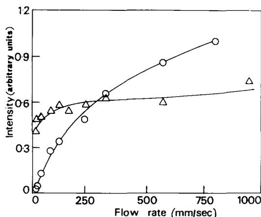
Figure 3 Transmitted light intensities of sodium alginate solution under flow (○) and calcium alginate gel fibre (△) as a function of flow rate in the tube. The intensities are normalized by that of the sensitive tint plate (530  $\mu\text{m}$ )
