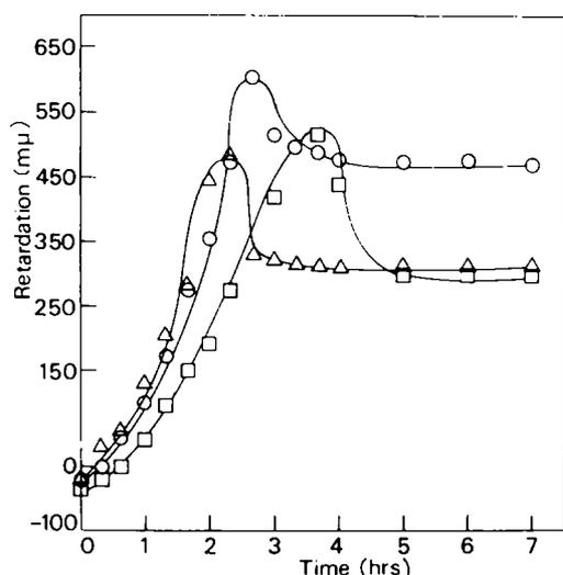
Figure 10 Retardations of gel fibres obtained at various extrusion rates as a function of drying time: ( $\Delta$ ) 8; ( $\circ$ ) 32; ( $\square$ ) 160 mm s<sup>-1</sup>
