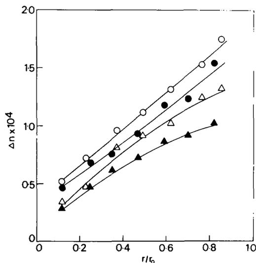
**Figure 7** Birefringences of transverse (circles,  $\Delta n \equiv \Delta n_{yx}$ ) and longitudinal (triangles,  $\Delta n \equiv \Delta n_{zx}$ ) cut sections of gel fibre obtained at an extrusion rate of  $19.5 \text{ mm s}^{-1}$  as a function of  $r/r_0$ . The closed and open symbols represent the 'unwashed' and 'washed' specimens, respectively
