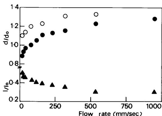
**Figure 2** Diametric expansion (circles) and longitudinal shrinkage (triangles) ratios of extrudates in  $\text{CaCl}_2$  solution as a function of flow rate in the tube. The open and closed symbols represent the values immediately after and 1 day after extrusion, respectively; the diameter  $d_0$  is 2 mm and the length  $l_0$  is defined as the length derived by dividing an extruded volume by the cross-sectional area of the tube;  $d$  and  $l$  refer to extrudates
