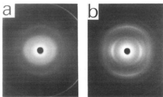
**Figure 12** Wide-angle X-ray diffraction patterns of (a) calcium alginate xerogel fibre (flow rate  $9.5 \text{ mm s}^{-1}$ ) and (b) the corresponding acidified fibre
