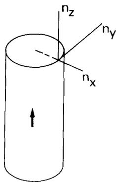
**Figure 6** Co-ordinate system of refractive indices  $n_x$ ,  $n_y$  and  $n_z$  relating to the cylinder-shaped gel fibre of calcium alginate. The arrow indicates the total flow direction
