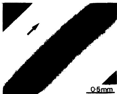
Figure 4 Typical features of a polarized optical micrograph of a cylinder-shaped calcium alginate gel fibre. The arrow indicates the total flow direction
