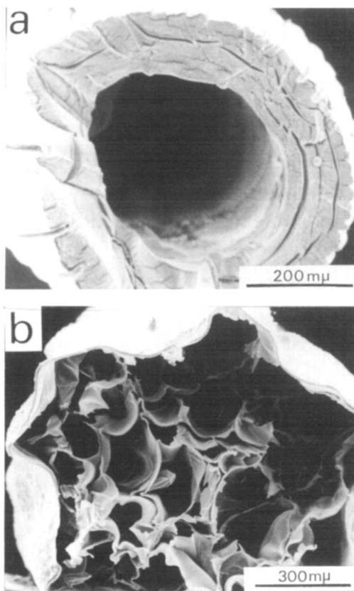
**Figure 9** Scanning electron micrographs of vacuum dried gels soaked in water for (a) 1 min and (b) 2 h before drying
