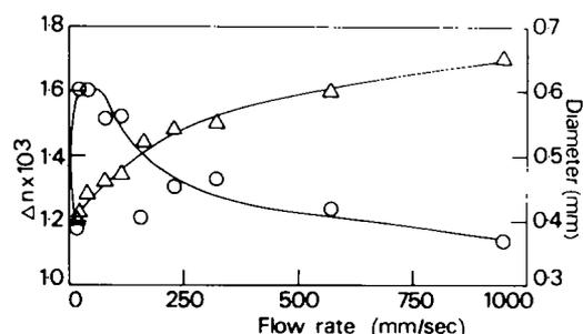
Figure 11 Birefringence ( $\circ$ ) and diameter ( $\Delta$ ) of xerogel fibres as a function of flow rate in the tube. The specimens were those obtained by drying the 'washed' gels of constant length at room conditions
